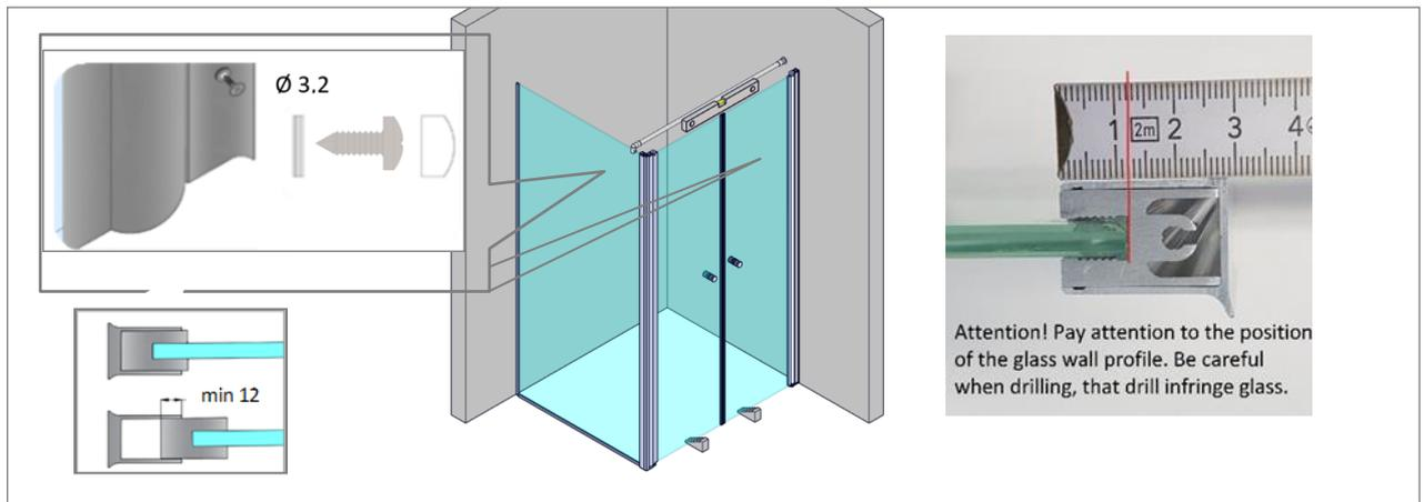
Attach the upper cab bracket as indicated. The distance from the edge of the wall profile to drill holes in the center is 50-55mm.
